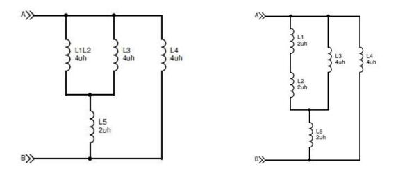
First complete the series Inductors, then parallel. Here, L1 and L2 are added together, then with L3
